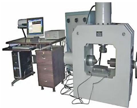
Figure 4. YZW30 computer-controlled rock stress direct shear apparatus
