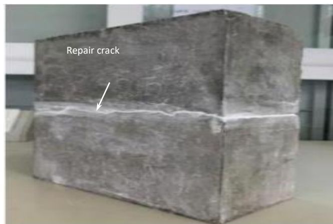
Figure 5. MICP cemented joint specimen
