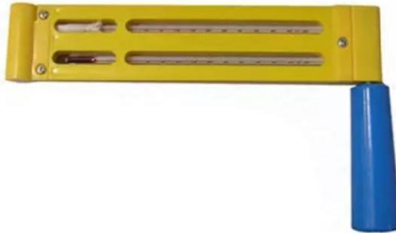
Figure .4: Sling/Whirling Psychrometer
