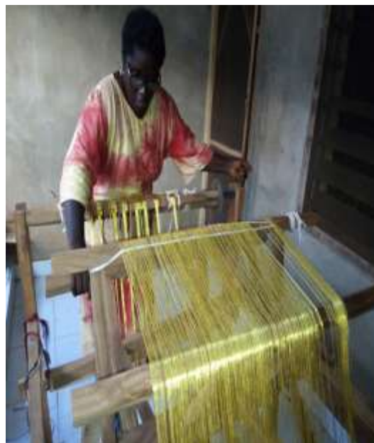
Figure 7. VictoriaOgundipe, Beaming the Warp Yarns on the Roller, 2018, (Photograph – Abeni Ayoola.) Osun State.
