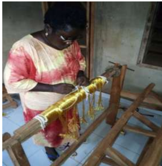
Figure 8. Victoria Ogundipe, Securing the Warp Yarns, 2018, (Photograph –Sola Ojo) Osun State.
