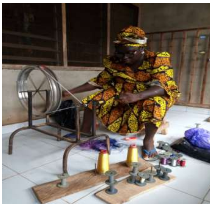
Figure 3. Victoria Ogundipe, Transferring yarn from Cone to Bobbins with the aid of Winding Wheel, 2018, (Photograph – Abeni Tayo) Osun State.
