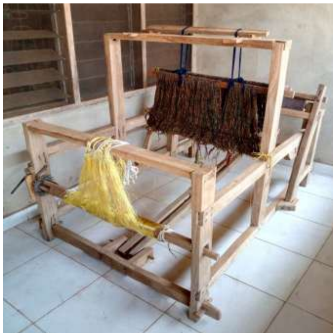
Figure1. Broad Plain Loom, 73 / 42 / 52 cm, 2016, Photograph – Victoria Ogundipe, Ilesa, Osun State
