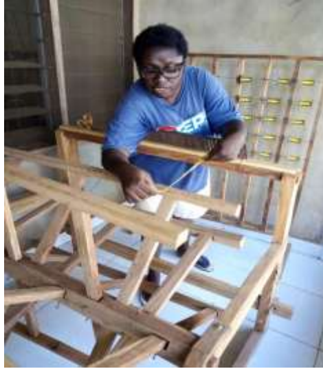
Plate viii. Victoria Ogundipe, Transferring yarn from Cone to Bobbins with the aid of Winding Wheel, 2018, (Photograph – Abeni Ayoola) Delta State University.
