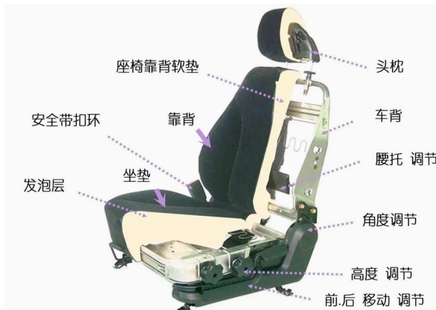
Figure 5: Schematic diagram of adjustable lumbar support mechanical structure
